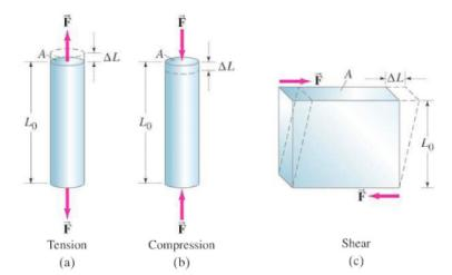
FIGURE 9-22 The three types of stress for rigid objects.
